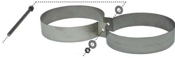
6) Place another flat washer onto the bolt from the front of the cylinder and then using a spanner to hold the bolt's end nut and another to turn the aircraft nut onto the bolt. DO NOT FULLY TIGHTEN AT THIS STAGE.
